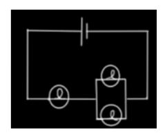
The first globe is in series which means that all the current flows through the first globe and then the current splits into two. Whereby, half flows into the second and the other half flows through the third. 1.9mA and 1.8mA is flowing through the second and third globe.
