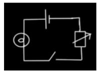
We can change resistance. When you close the switch, it allows the current to flow.
