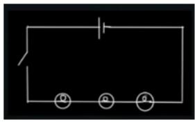
The 12V provided by the power supply will be used up by the three components. If we add the voltage drop between each of the components it should add up to almost 12V. it won't be exact because the wires have some resistance.
