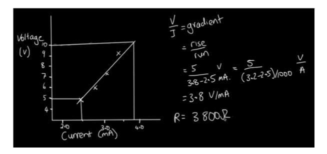
The relationship between V and I is called ohms law. We can use this law to calculate the voltage, current or resistance in a circuit.
