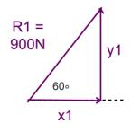
Step 1. Resolve into horizontal and vertical components
