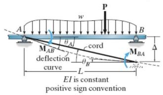
DOF for the general beam is  $\theta_A$ ,  $\theta_B$ ,  $\psi$  (=  $\Delta/L$ )
