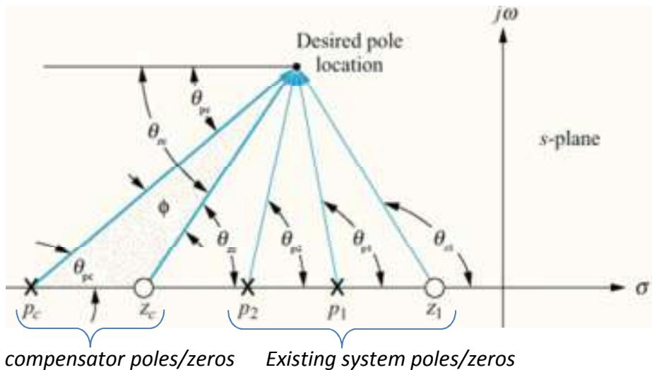
As can be seen, there are infinitely many choices of  $p_c$  and  $z_c$  that have the same required angle difference between them. Angle bisection method can be used to find ideal locations:
