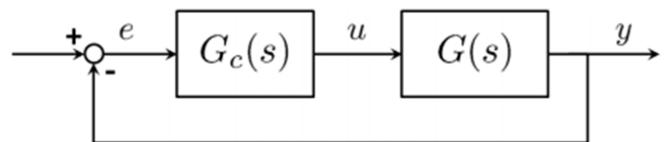
$$u(t) = K_p e(t) + K_i \int_0^t e(\tau) d\tau + K_d \frac{de}{dt}(t) = K_p \left\{ e(t) + \frac{1}{T_i} \int_0^t e(\tau) d\tau + T_d \frac{de}{dt}(t) \right\}$$
