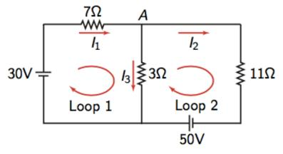
The current through point A gives:  $I_1 - I_2 - I_3 = 0$ The voltage drop around Loop 1 gives:  $7I_1 + 3I_3 = 30$ The voltage drop around Loop 2 gives:  $11I_2 - 3I_3 = 50$
