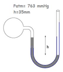
The right hand side is open whereas the left-hand bulb contains the unknown gas (exerting an unknown pressure)
