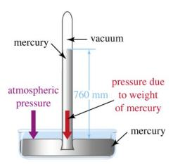
The pressure from the atmosphere is pushing down the mercury in the dish. However the downward pressure of the mercury (due to its weight) is pushing upwards i.e. the level of mercury wants to rise. Once the two pressures are equal (i.e. at a height of 760mm), the level of mercury can no longer rise. This gives a relative indication of the pressure that exists in the atmosphere (atmospheric pressure)
