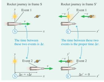
**VISUALIZE FIGURE 36.22** shows the two events as seen from the two reference frames. Notice that the two events occur at the *same position* in S', the position of the rocket, and consequently can be measured by *one* clock.
