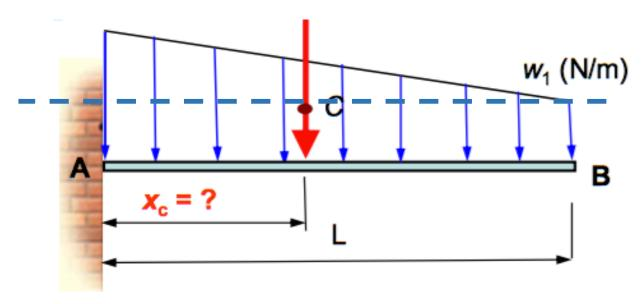
Step 1: divide the system into 2 simple shapes → a triangle and a rectangle
