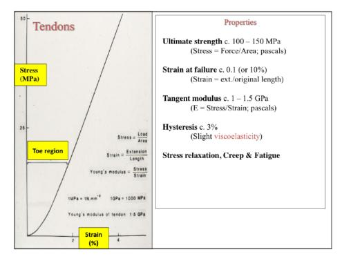
Elastic - immediately get stress in response to constant load. With collagen, a constant load results in increased stretch (strain goes up) and overtime deformation increases [creep].
